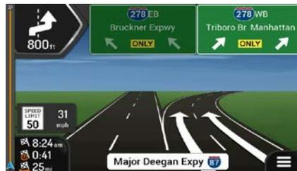
**Cause:** If you are approaching a freeway exit or a complex intersection and the needed information exists, the map is replaced with a 3D view of the junction. The lanes you need to take are displayed with arrows.
