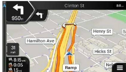
There is a field in the top left corner displaying the next maneuver. Both the type of the maneuver (turn, traffic circle, exiting freeway, and so on) and its distance from the current position are displayed.
