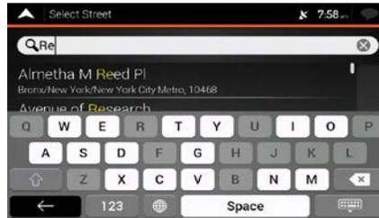
**Cause:** Advent Generation II has a smart keyboard for address search, which means that only those buttons are active that can be used to type a name that is available on the map.
