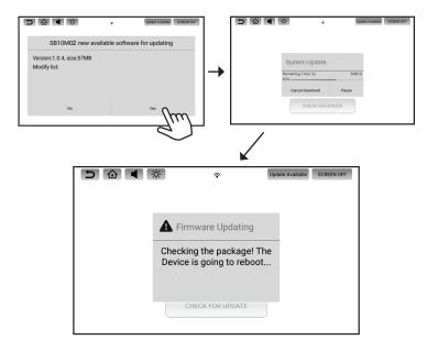
**NOTES**: <u>Do not disconnect power from the monitor during the update process</u>. Once the software download is complete, the system will check the downloaded files and then begin the update process. When the update process is complete, the monitor will return to the standby mode. Press the Power Button to turn the monitor on and resume operation.
