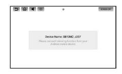
4. After a few seconds, the Receiving monitor's Device Name will be displayed under "Available Device" on the Transmitting Monitor.
