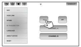
Select the desired Channel (A or B) for the IR Transmitter. It is recommended to select Channel A for one monitor and Channel B for the other monitor.
