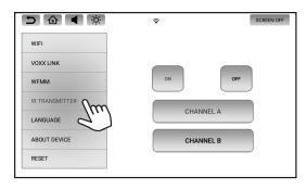
3. Touch the **ON** or **OFF** button to turn ON or OFF the IR Transmitter.
