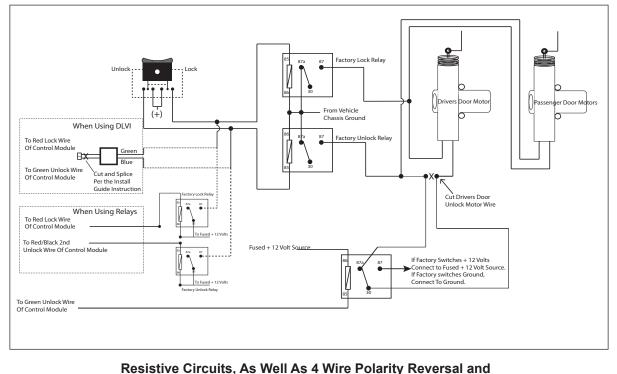
5 Wire Alternating 12 Volt Door Lock Control Circuits
