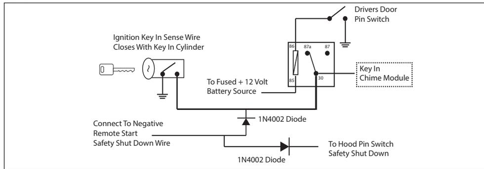
To connect to the key in sensor as shown in method 1:
