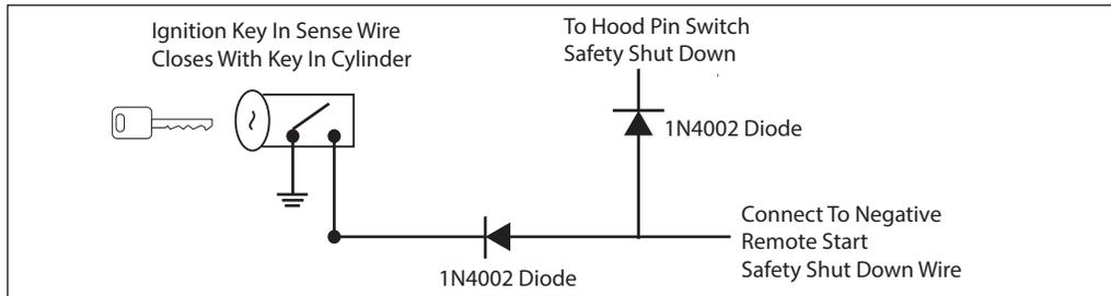
To connect to the key in sensor circuit as shown for method 2:
