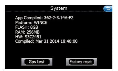
GPS test will identify how many satellites are being received. Note the antenna is located in the mirror housing. Do not place any object over the mirror housing or on the windshield above the mirror or this will block the signal.
