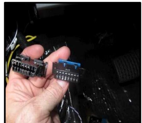
3. Locate the green and black wires on the back of the factory OBD connector (you can use the extension OBD harness as reference of the wire locations). Connect a T-Taps to each of the green and black wires. Connect the white wire to the green wire and connect the purple wire to the black wire. You may also use other types of connectors or solder the wires, whatever your preference. (Figure F3a-b)
