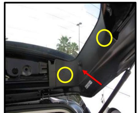
6. Loosen rubber harness gasket from between the vehicle and the liftgate. (Figure B6)
