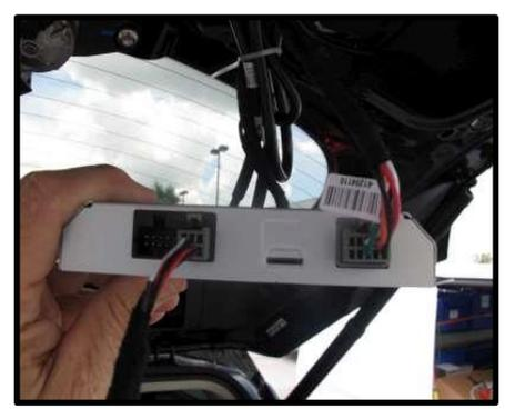
2. Mount Control box permanently. Use wire ties to clean up all routing making sure cables do not rattle or interfere with any other vehicle parts or operation. (Figure G2)
