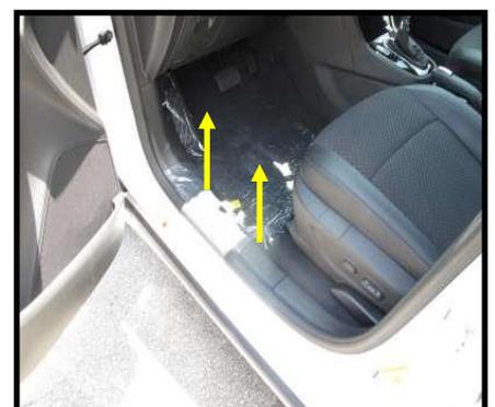
10. Using an NRT pry the driver side IP panel off.
