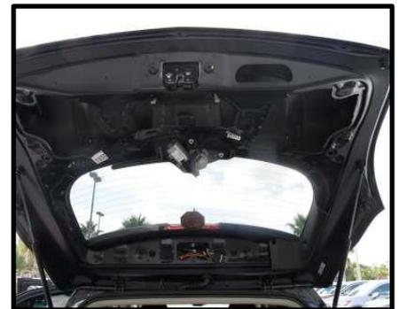
5. By hand loosen 2 metal clips on right-side trim panel from tailgate. **DO NOT try to remove the center hanger, it is a onetime press in part.**
