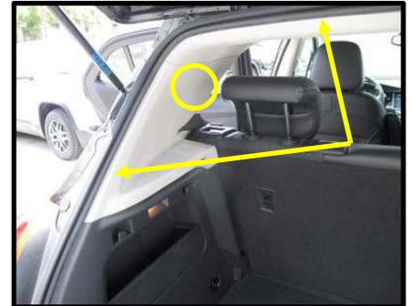
8. Loosen rear driver side rubber gasket and remove lower door sill panel. (Figure B8)
