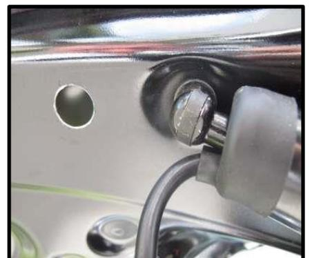
4. Route strut cable through hole and push bushing into the hole. Continue routing cable into liftgate area towards control module position.
