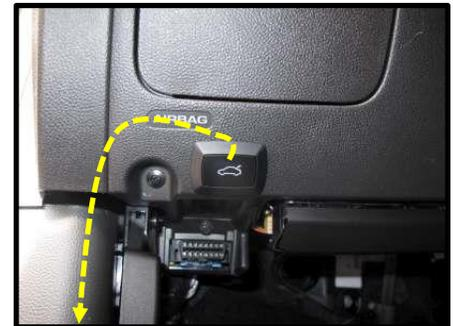
6. Install BUS Box to lower side wall with supplied double side tape. Route and plug in switch wires and OBD wires into BUS box. Connect BUS box cable to Main harness. (Figure E6a-b)
