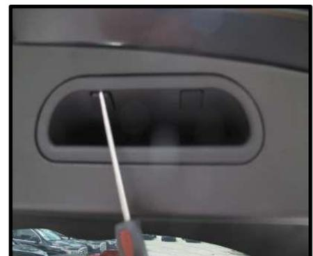
3. Place template onto rear liftgate cover with template aligned with pocket opening. Hold template in place with tape. Using the 16mm drill bit (supplied), drill at center point marked. Drill pilot hole through plastic and metal. Drill 16mm
