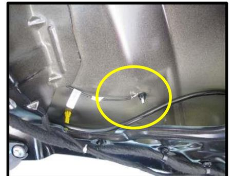
7. Now route main harness into vehicle. Continue routing main cable through gasket between headliner and over to rear side panel. Continue behind side interior panel making sure harness is routed over upper clip. **DO NOT route harness where it may interfere with seat belt.**
