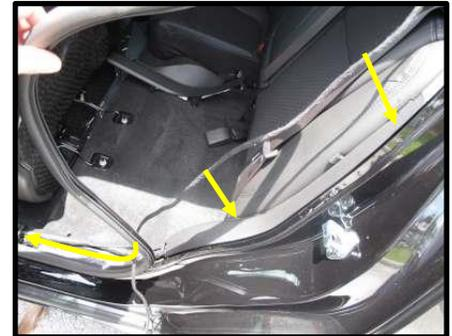
9. Continue routing cable forward tucked under lower B-pillar panel and into driver side sill area. (Figure E8)
