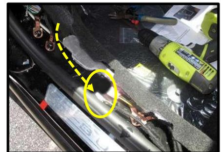
7. Locate Main power supply connector inside fuse box opening (Red-Black wires/ Blue connector). Connect X-large Tap connector (PBB580008100) to the Red wire. Screw Tap cover into place. Route cable and ground eyelet down to door sill. Connect ground loop eyelet to the factory studs shown. Connect power connector to main harness. (Figure E7a-e)
