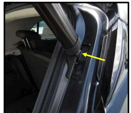
3. Using supplied drill bit, drill 16mm hole through side wall of the tailgate approximately 40mm or 4cm rear of strut mount. **CAUTION: check drill**
