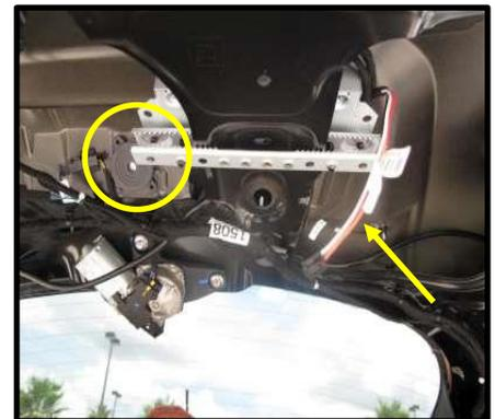
4. Route the main harness through the rubber gasket. Allow enough harness to extend towards rear to reach Control box. **NOTE: use a wire puller to pull harness through gasket. Protect harness connectors by taping over them so they pass through easier.** (Figure E4)
