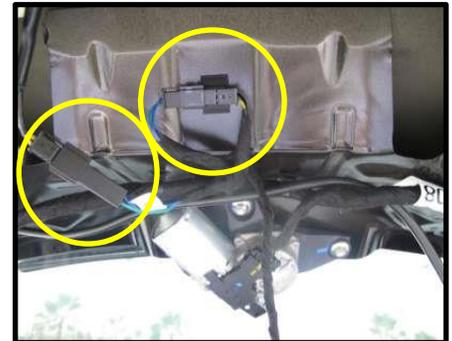
2. Locate Tailgate latch connector (Blue-Grey Cable/ Black connector). Disconnect the connector and insert Lock T harness of 3110122001019. Continue routing cable towards Control Box. (Figure E2a-b)
