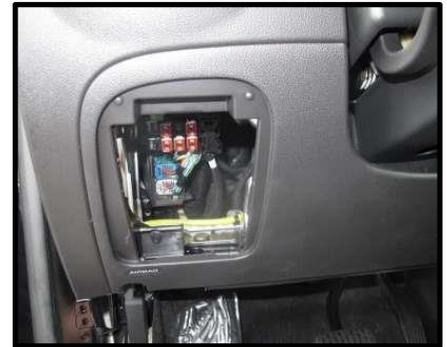
11. Using a #2 Phillips screwdriver remove the screw holding the OBD bracket. Using a 7mm socket remove screw holding OBD bracket.
