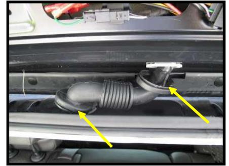
7. Loosen rubber gasket and left rear trim panel of the tailgate opening. (Figure B7)
