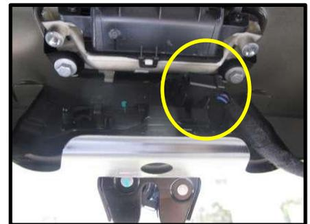
3. Mount buzzer and harness 1901454235500 to rear tailgate in location that will not interfere with tailgate trim panel. This cable also plugs into rear switch. (Figure E3)
