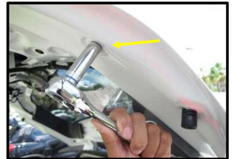
2. Install new electric struts into place making sure that the strut marked **RIGHT** is on the Passenger side. Push strut socket onto strut ball with harness up and facing the tailgate. Continue installing Driver's side strut. (Figure C2a-c)
