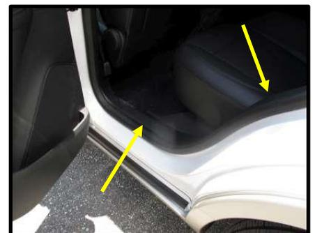
9. By hand remove twist nut from upper front corner of the driver lower door sill panel. Pull up and remove lower panel. (Figure B9a-b)
