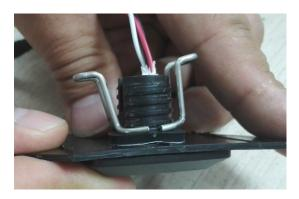
19. Mount the open/close button and secure with the nut. Connect to the main control module.
