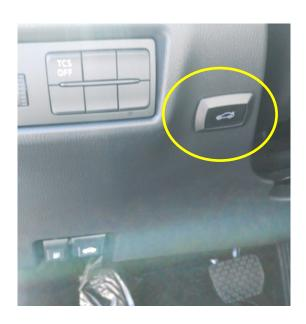
21. IMPORTANT: Prior to closing, ensure door panel is re-installed. Manually close the lift gate to initialize the Power Lift Gate System. Function test the system to verify proper operation.
