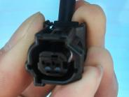
10. Locate the OEM power latch. Disconnect the OEM connector, and connect our T-Harness in line with the power latch assembly.
