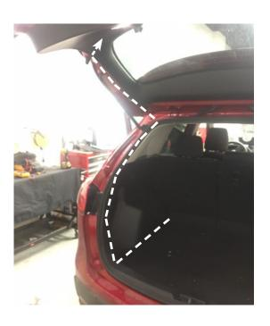
15. Route the main wiring harness through the OEM grommet and into the lift gate. Use a fish tape to help in pulling the harness through the factory wiring boot. Exercise care not to damage the harness or connectors when pulling the harness through the boot. Route the main wiring harness along the factory wiring harness to the main control module and connect to the main control module.
