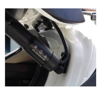
7. Remove the factory rubber grommet. Route the wiring harness through the hole and into the lift gate, seating the included grommet on the harness into the cavity from where the factory grommet was removed. Repeat for the opposite side.
